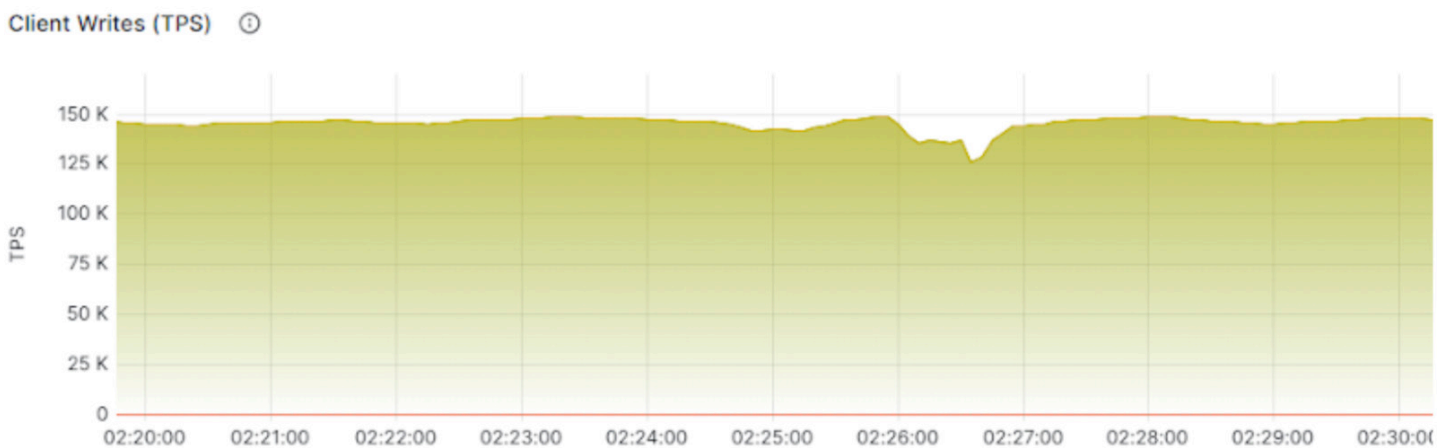
Figure 15.2 - "Zoom in" of Aerospike during a node failure (as it's hard to notice): no loss of service with Min dropping from 149K to 126K.
