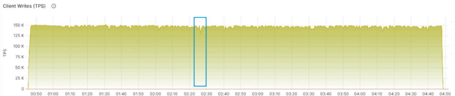
Figure 15.1 - Aerospike during a node failure: no loss of service.
