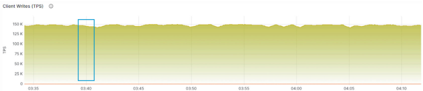
Figure 17: Quiescing an Aerospike node at 03:40 has no impact on throughput.
